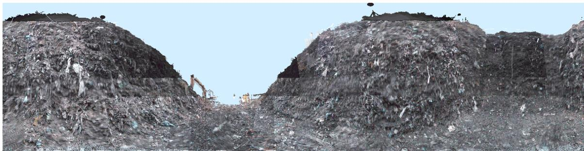
Fig. 1: Panoramic view of the excavation produced by merging the laser scanning data.
