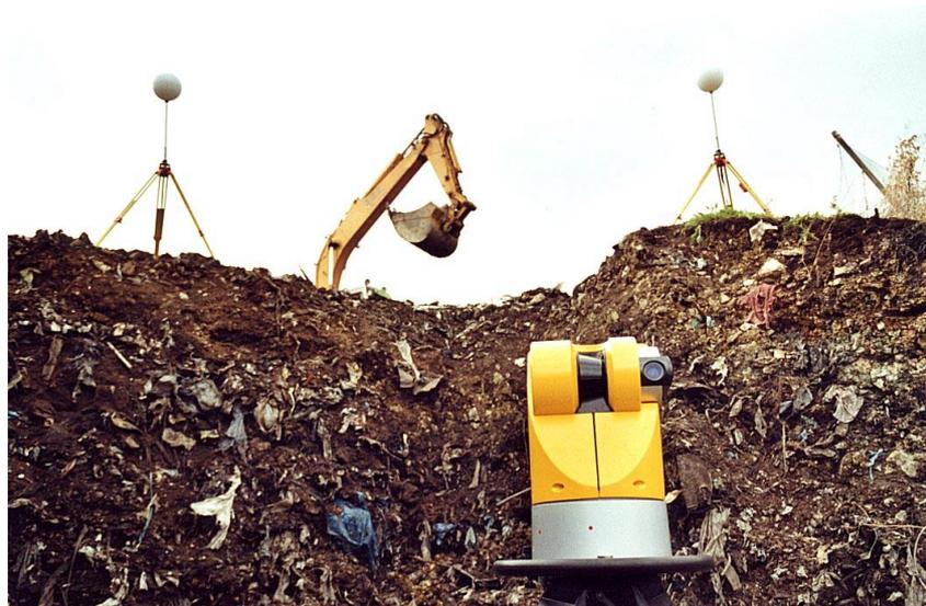
Fig. 2: The laser scanner at work. On the top two reference spheres are visible.
